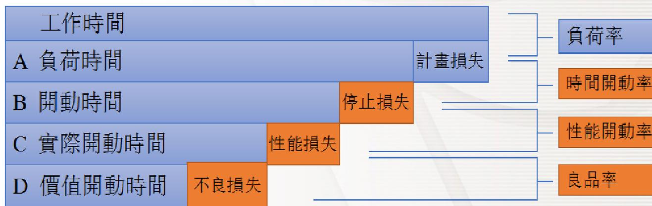
$$\text{OEE} = \text{時間稼動率} \times \text{性能稼動率} \times \text{良品率} = B/A * C/B * D/C$$
